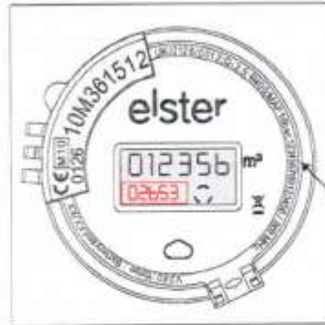
Figure 17 V200 & V210 Shroud Markings of Electronic Register with Radio Output.
