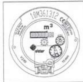
Figure 16 V200 and V210 dial face showing position of Reed Switch Sensor
