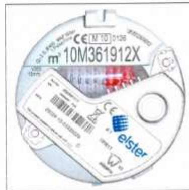
Figure 46 Sketch of inductive sensor mounted on a MSII polymer cased register's shroud.
