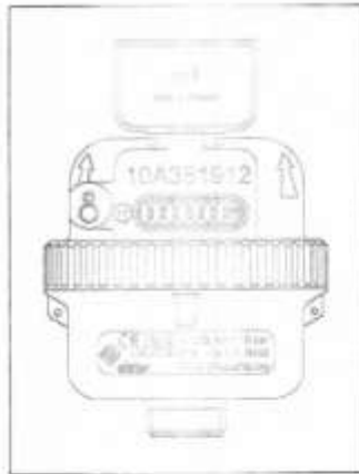
Figure 35 V110 serial number and verification marks
