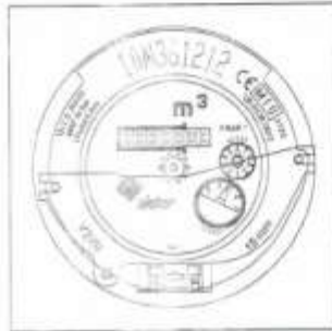
Figure 12 V200 and V210 dial face showing position of Inductive Sensor
