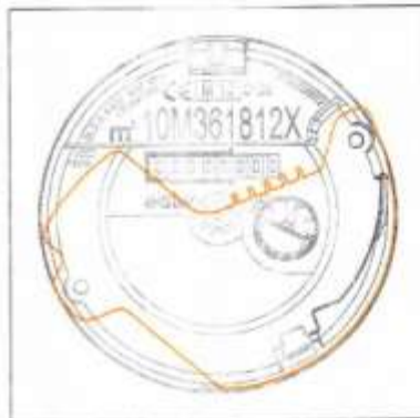
Figure 45 Outline of inductive sensor position on a MSII copper can register's shroud.
